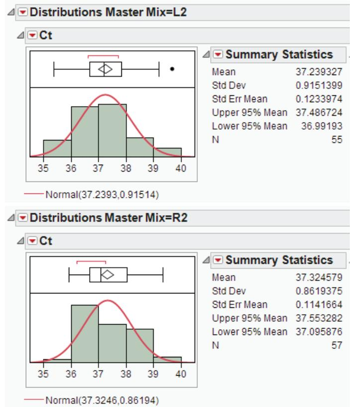
**Figure 11. Distribution of RNase P  $C_t$  values obtained from 2 copies/ rxn of CEPH gDNA.** Data from three PCR setups were combined (20 technical replicates each, total n = 60). Data are displayed using the JMP 10 Statistical Software package (SAS Institute Inc.) for a single, representative master mix lot. Reactions that did not amplify were considered to have 0 copies of CEPH gDNA, a result of sampling error near the digital concentration range.
