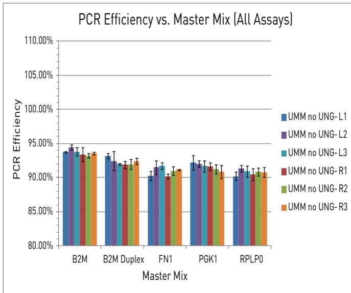
Figure 6. PCR efficiency values for each gene expression assay, calculated from the slope of the mean  $C_t$  vs.  $\log(\text{conc.})$  plot. Each assay exhibited consistent efficiencies between lots of Universal PCR Master Mix, No AmpErase<sup>®</sup> UNG (differences <2%).
