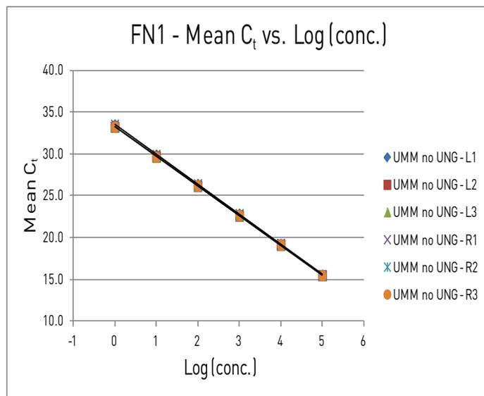
Figure 1A. FN1 (Hs00277509\_m1) mean  $C_t$  values plotted across 5 logs of cDNA sample for all six lots of Universal PCR Master Mix, No AmpErase® UNG.
