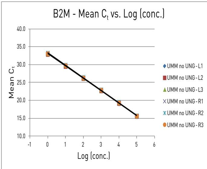
Figure 4A. B2M (Hs00363670\_m1) mean  $C_t$  values plotted across 5 logs of cDNA sample for all six lots of Universal PCR Master Mix, No AmpErase® UNG.
