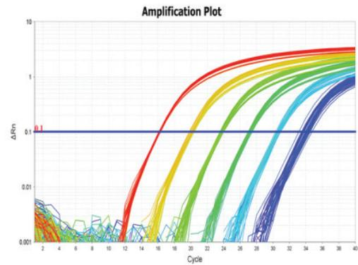
Figure 2B. PCR amplification plot overlaying technical replicates from all six master mix lots at each concentration point.
