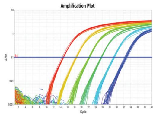
Figure 3B. PCR amplification plot overlaying technical replicates from all six master mix lots at each concentration point.
