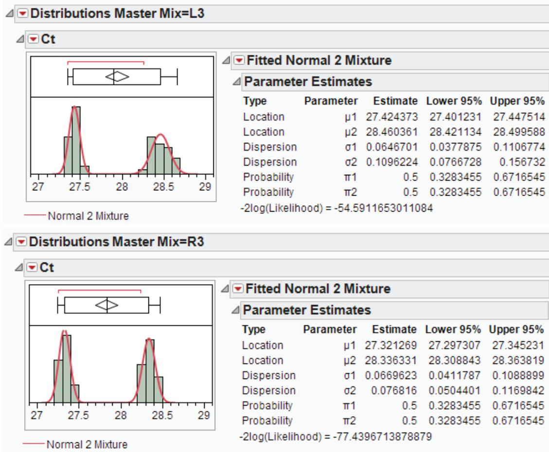
Figure 12. Distributions of RNase P  $C_t$  values obtained from 1,600 and 800 copies/rxn of CEPH gDNA. Data from three PCR setups were combined (10 technical replicates for each concentration, total  $n = 30$ ). Data are displayed using the JMP 10 Statistical Software package (SAS Institute Inc.) for a single, representative master mix lot.
