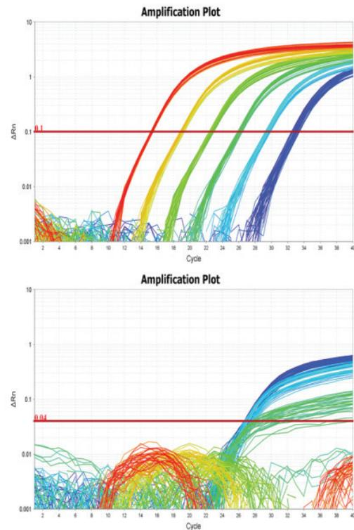
Figure 5B. PCR amplification plot overlaying technical replicates from all six master mix lots at each concentration point and for the exogenous IPC (bottom). Note that at high concentrations the B2M assay out-competes the exogenous IPC, accounting for the observed variability in the IPC amplification plot.
