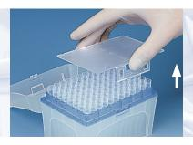
Remove the transfer aid from the mounting plate. Finished – all without tip contact!
