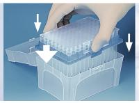
Insert the filled tip-tray perpendicularly from above into the previously sterilized TipBox until it locks into place.
