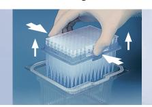
Press the long sides of the transfer aid together, and continue pressing them together while withdrawing the tip-tray. Ensure that the holding straps for the transfer aid are correctly positioned.
