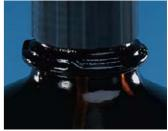
Valve block (45 mm) and included adapters (32 and 40 mm) match the threads of the most common reagent bottles.
