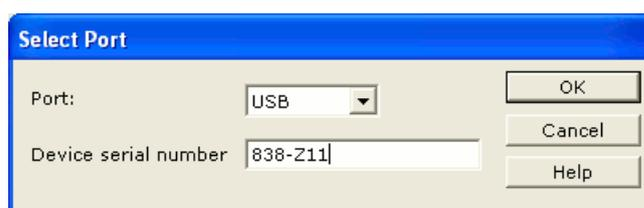
3. Select the serial communications port (COM 1–9) or USB port that the instrument is connected to from the **Port** list. When USB is selected, the *Device serial number* field can be left empty. Click **OK**.
