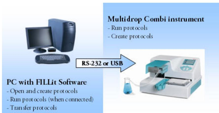
Figure 1-1. Operation principle
