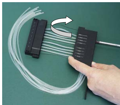
Figure 5-46. Precalibrating the dispensing cassette
