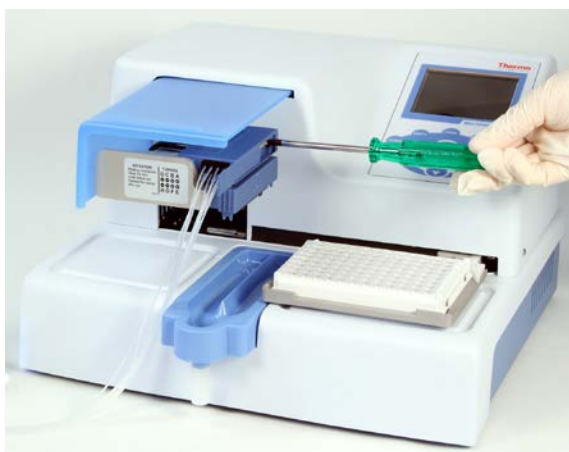
Figure 6–50. Screwing a calibration screw according to the calibration results
