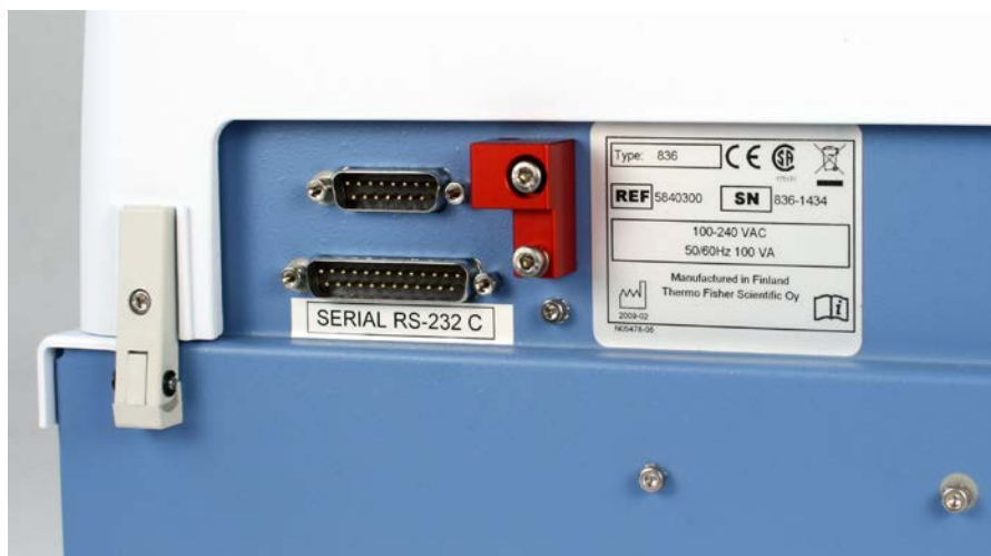
Figure 3–7. Transport lock storage
