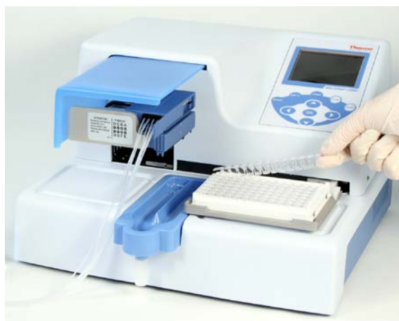
Figure 6–49. Removing the filled microstrip to be weighed
