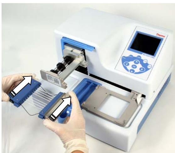
Figure 4–11. Inserting the dispensing cassette
