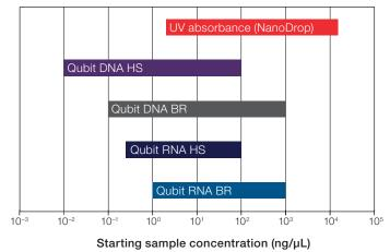
Figure 3. Comparison of sample concentration ranges for the Qubit assays and UV absorbance measurements using the NanoDrop Spectrophotometer.
