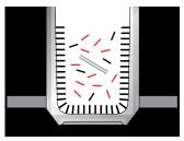
2. Buffer, dNTP's, Taq DNA polymerase, template and primers are added to a well containing the covalently bound primer. The amplification is semi-asymmetric since the relation between the bound and the unbound primer is 1:8.
