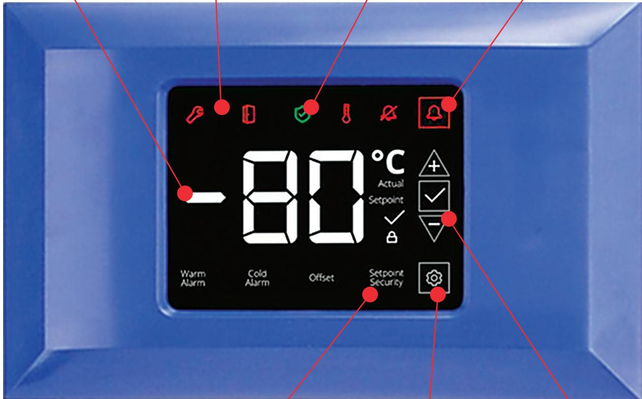
'Setpoint Security' allows you to set a three-digit numeric code required for any settings changes
