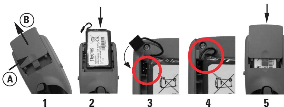
1. Open the battery lid (press (A) and slide (B)).
