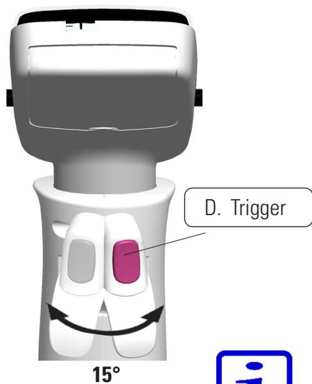
**D. Trigger:** The index finger operated trigger is used to aspirate and dispense liquid. It is also used to initiate mixing. The trigger and finger rest can be rotated 15 degrees in both directions to ensure an optimal pipetting position.
