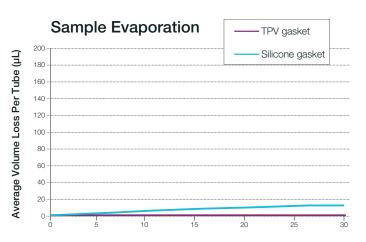
Figure 1. Average sample evaporation at room temperature in tubes with either TPV or silicone gaskets/closures.
