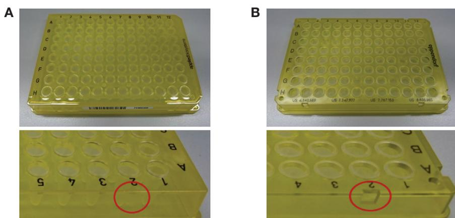
**Figure 4. Comparison of PCR plates.** (A) MicroAmp EnduraPlate full-skirted plate, with a view of the skirt in front of well A2. (B) twin.tec PCR plate, with a view of the robotic slot in the skirt in front of well A2.
