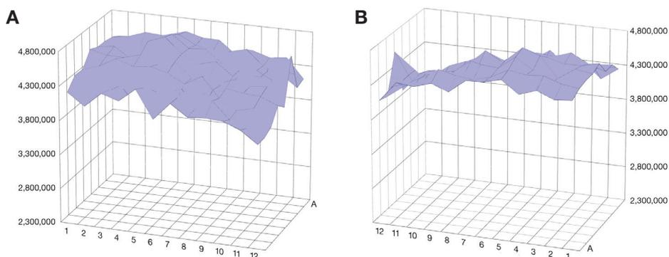
**Figure 2. Fluorescence intensity surface plots for the MicroAmp EnduraPlate full-skirted plate with 10  $\mu$ L reactions.** Data are shown for the (A) front and (B) back orientation of the plate.
