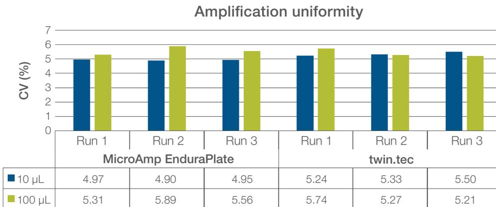
Figure 1. Amplification uniformity in full-skirted 96-well PCR plates on the ATC, as measured by CV.
