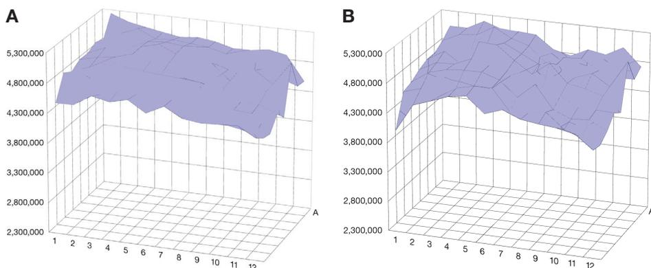
**Figure 5. Fluorescence intensity surface plots for 100  $\mu\text{L}$  reactions.** Data are shown for (A) MicroAmp EnduraPlate and (B) twin.tec PCR plates.
