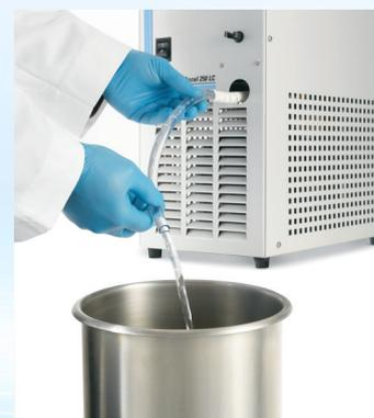
Flexible fill tube on the front panel enables unit to be drained quickly.
