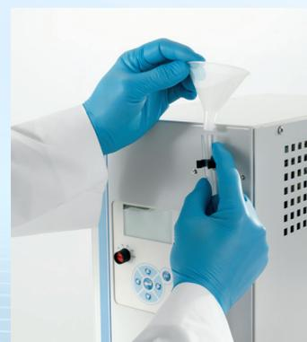
Site tube on the front of the unit allows for quick indication of the fluid level.
